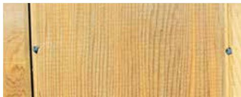
EXAMPLE OF SHRINKAGE IN A 1/2" THIN BOARD.
